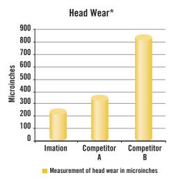
\* Head wear measured as the width of wear mark in a ferrite bar after running 1,700 feet of tape over the ferrite bar at 5 oz. tape tension.
